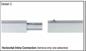
Each extrusion contains a numbered Remove only (1) setscrew when disassembling. Replace setscrew in extrusion after assembling it. Before packing, replace setscrew in extrusion to avoid losing it.
