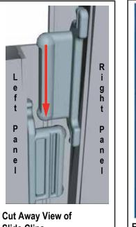
Slide Clips Components connect together by aligning them and sliding downward connecting clips together.
